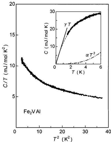
FIG. 5. Specific heat divided by temperature,  $C/T$ , versus  $T^2$  measured for  $\text{Fe}_2\text{VAI}$ . The inset shows the  $C$  versus  $T$  plots, and the dash-dotted line represents the lattice contribution  $\alpha T^3$  ( $\alpha = 0.031 \text{ mJ/mol K}^4$ ) for  $\text{Fe}_3\text{Al}$  (Ref. [17]). The specific heat is approximately of the form  $C = \gamma T$  at sufficiently low temperatures.
