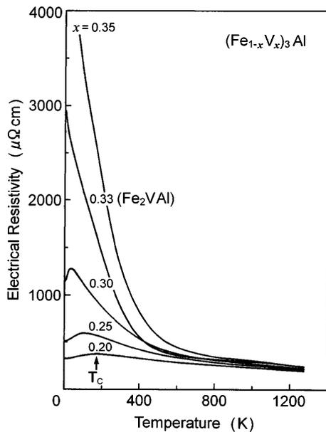
FIG. 3. Temperature dependence of electrical resistivity in  $(\text{Fe}_{1-x}\text{V}_x)_3\text{Al}$  with  $0.20 \leq x \leq 0.35$ . The curve for  $x = 0.20$  is the same as that shown in Fig. 2, and the arrow indicates the Curie temperature  $T_c$ . Note that  $\text{Fe}_2\text{VAI}$  ( $x = 0.33$ ) exhibits a semiconductorlike behavior.
