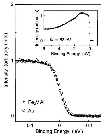
FIG. 4. Energy distribution curve of  $\text{Fe}_2\text{VAI}$  (dots) near the Fermi level in comparison with that of Au (open circles). A valence-band photoelectron spectrum of  $\text{Fe}_2\text{VAI}$  is also shown in the inset. All the spectra were measured at 40 K with an exciting photon energy  $\hbar\omega = 63$  eV.
