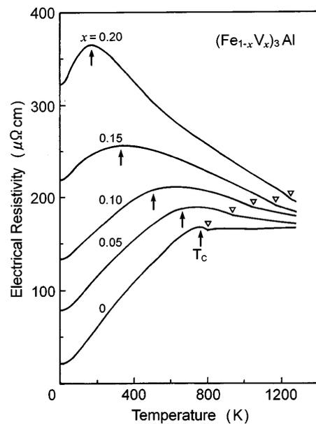
FIG. 2. Temperature dependence of electrical resistivity in  $(\text{Fe}_{1-x}\text{V}_x)_3\text{Al}$  with  $0 \leq x \leq 0.20$ . The arrows indicate the Curie temperatures  $T_c$ , and the open triangles indicate the  $D0_3$ - $B2$  transformation temperatures.
